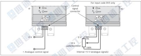
Figure 2-8 Control signal connection (self-powered unit without alarms)
