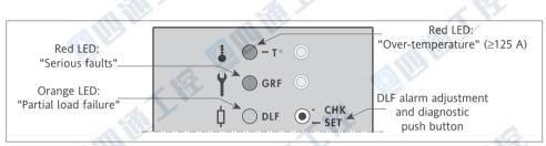
Figure 5-2 Layout of front panel LEDs with 'GRF' and/or 'DLF" option
