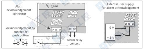
Figure 2-10 Typical alarm relay contact and external acknowledgement connections **2.3.2.5. Acknowledgement signal (ICO option)**
