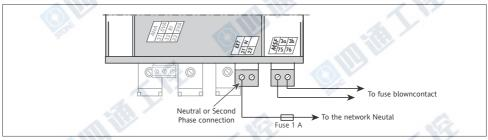
Figure 2-11 Connecting the supply neutral voltage
